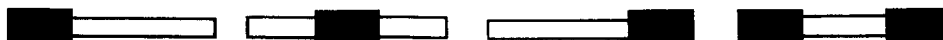
Fig. 1. Examples of MBOs; The dark area represent non-ionic segments, while the open area represent ionic segments. 3d
